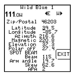
The arm angle, skew setting and APA number are also calculated and displayed at the bottom of the screen.
