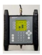
**Connections:** Coax cable connected from output port of DIRECTV SWM SL5s LNBF to top (SIGNAL IN) port of Super Buddy meter.
