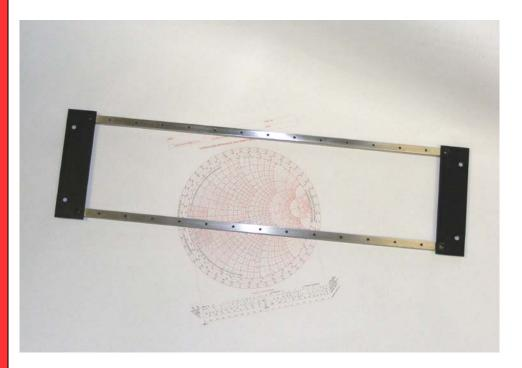
The **RFC-RM** is an accessory designed specifically for the **RF Cogs™** module series. Up to thirteen modules can be mounted into this sub-rack. The populated sub-rack can be readily mounted to a standard 19" equipment rack. The sub-rack and modules together occupy a 3U high space\*.
