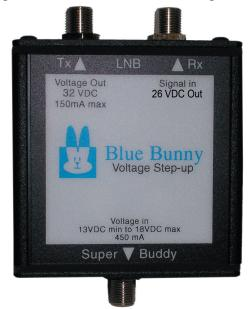
To satellite meter providing LNB power
