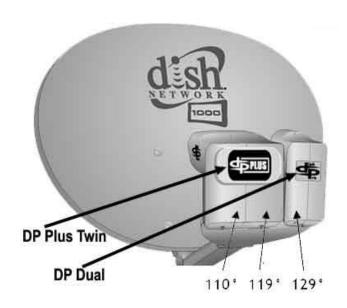
**Connections:** LNBs: DPP (110° and 119°) and DP (129°). Connect a coax cable from an output port of the DPP LNBF to the ODU / LNB port of the Al Turbo S2 satellite meter
