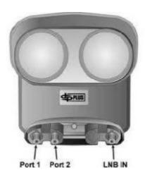
**Connections:** Coax cable connected from LNBF output port to the AI Turbo S2 satellite meter's ODU / LNB port
